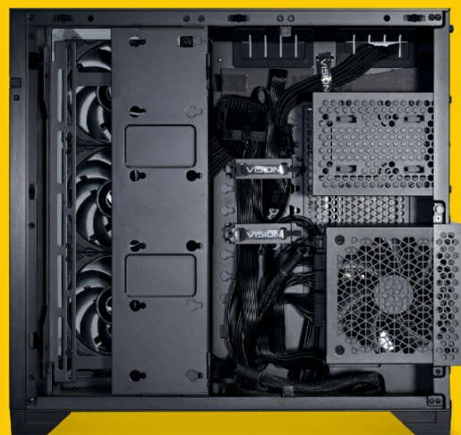
Image 5.1: A view of the second chamber, illustrating how cables are managed to maintain a clean appearance in the main chamber.
