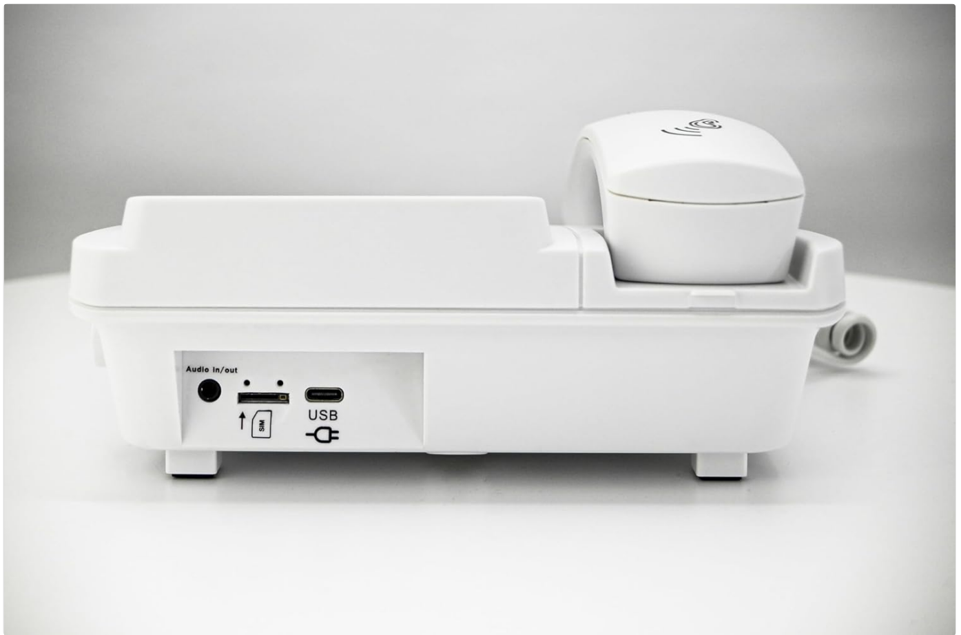
Figure 1: Rear view of the CL9000 phone, highlighting the SIM card slot and other connection ports like Audio In/Out and USB. This is where the 4G SIM card needs to be inserted.
