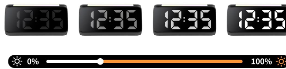
Figure 7: LED display color and brightness adjustment.
