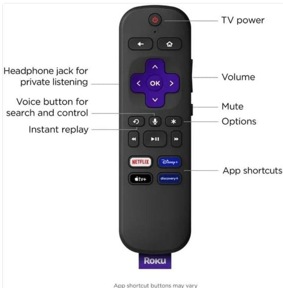
Figure 3: This image provides a detailed view of the Roku Voice Remote, labeling key features such as the TV power button, headphone jack, volume controls, mute button, voice button for search and control, instant replay, and dedicated app shortcut buttons.
