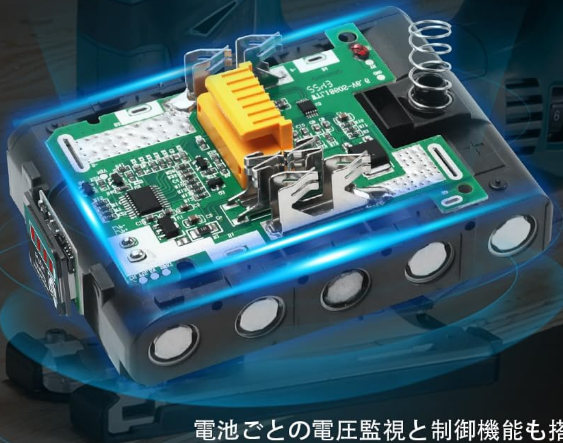
Image 5.2: Internal view of the battery, demonstrating its protective circuitry.
