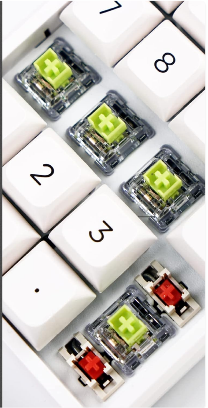
Figure 6.1: Detailed view of the Huano mechanical switches, highlighting their design and hot-swappable nature.
