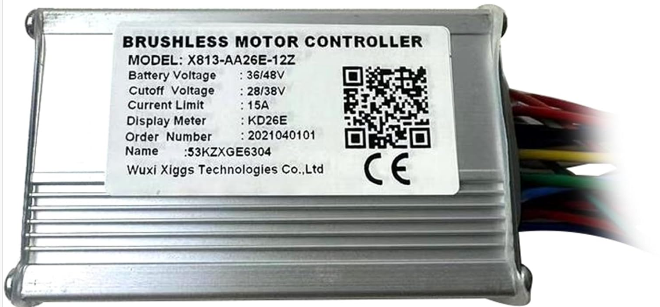
Figure 2: Close-up view of the controller's label, showing model and specifications.
