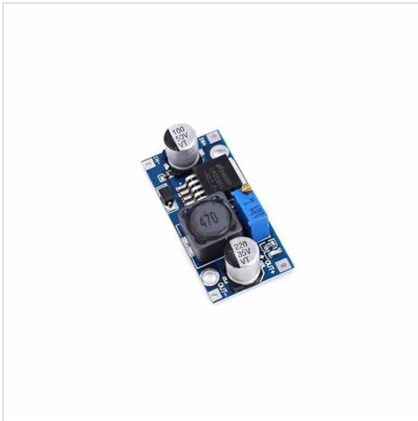
Figure 2.2: Angled view of the LM2596S Buck Converter module. This perspective clearly shows the input terminals labeled 'IN+' and 'IN-' on one side, and the output terminals 'OUT+' and 'OUT-' on the opposite side, facilitating connection identification.
