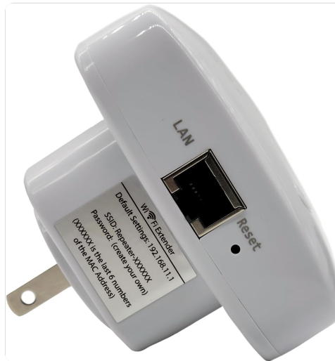
Rear view of the WiFi Extender, displaying the LAN port and the label with default settings and IP address.
