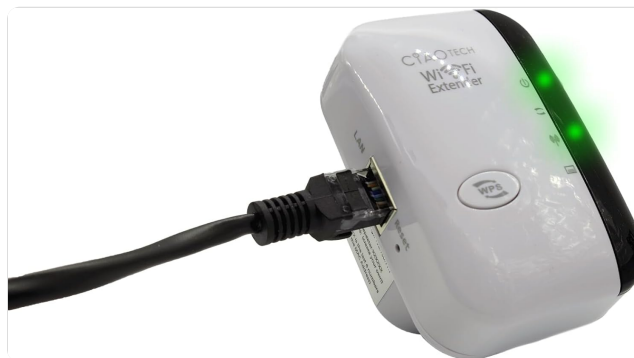
The WiFi Extender with an Ethernet cable connected to its LAN port, indicating a wired connection option.
