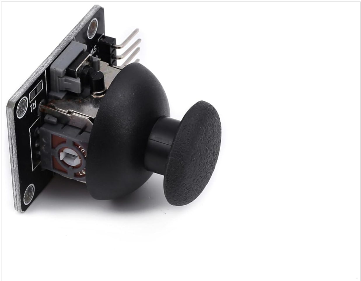
Figure 5.1: Angled view of the KY-023 Joystick Module, demonstrating the range of motion for the joystick lever.
