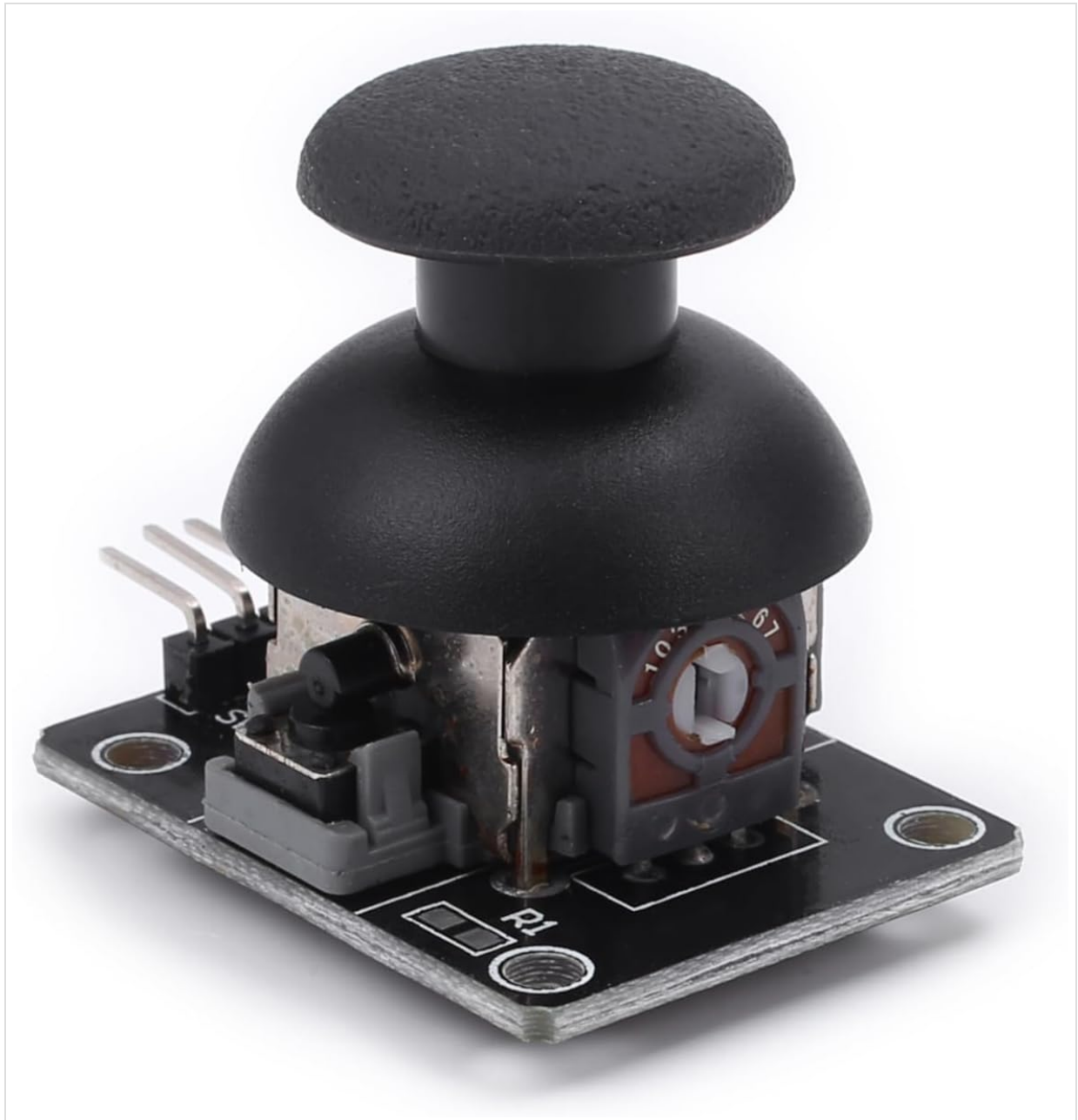
Figure 4.1: Side view of the KY-023 Joystick Module, illustrating the potentiometers for X and Y axis control and the R1 pads for the switch.
