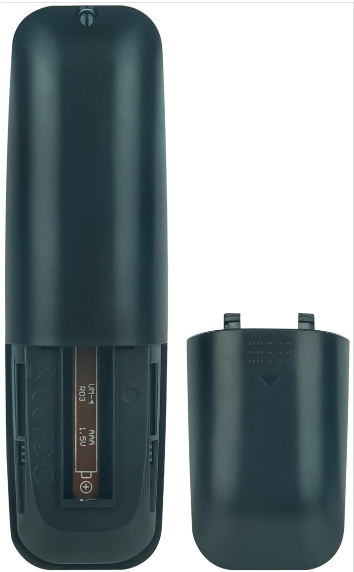
Image Description: The back of the remote control with the battery cover removed, showing the empty battery compartment designed for two AAA batteries and their polarity markings.
