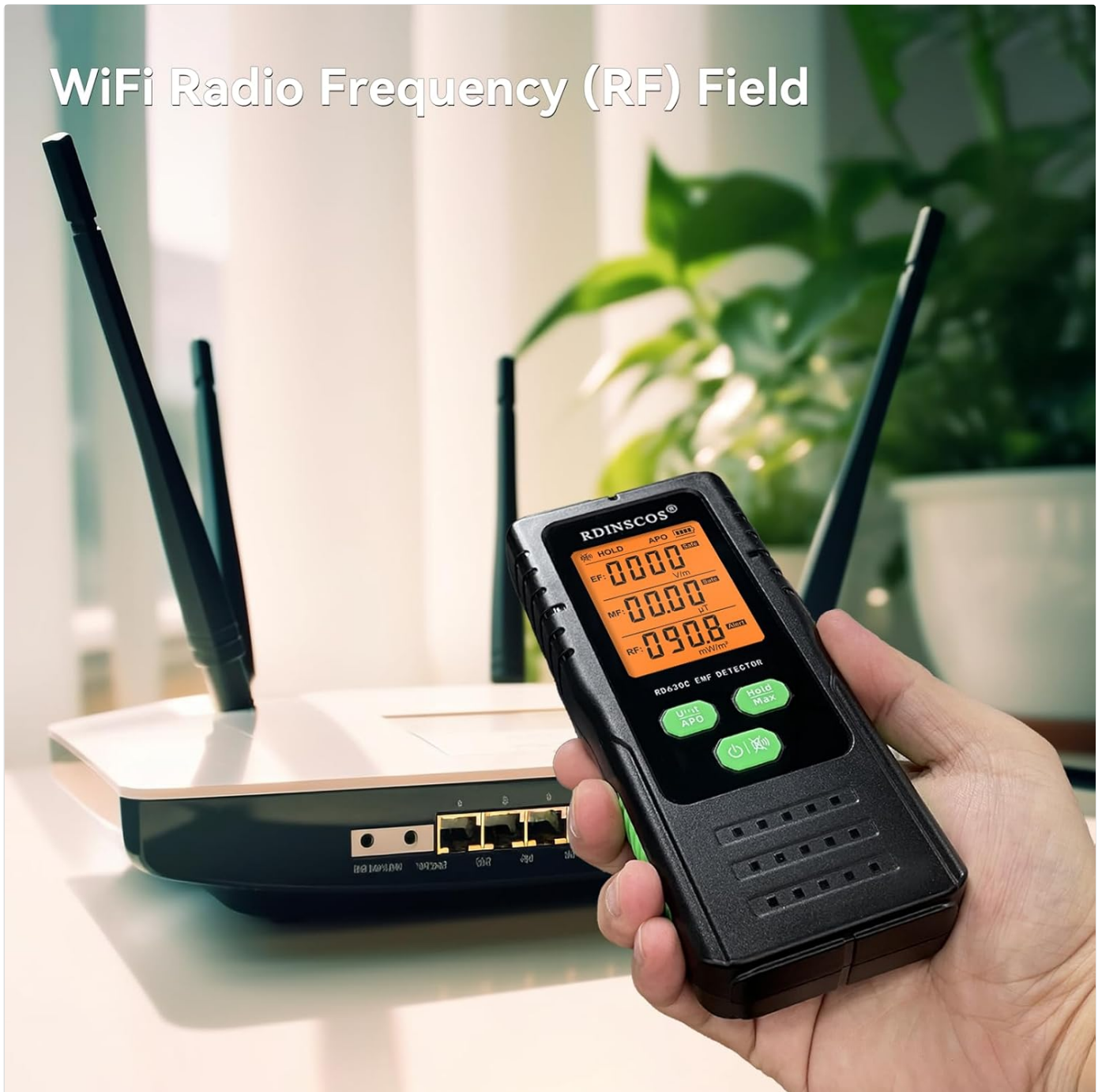
Figure 3: The RDINSCOS Digital EMF Meter RD630C being used to measure radiation near a Wi-Fi router. The screen displays readings for EF, MF, and RF, with the RF reading showing a yellow 'Alert' level, indicating moderate radio frequency radiation from the router.
