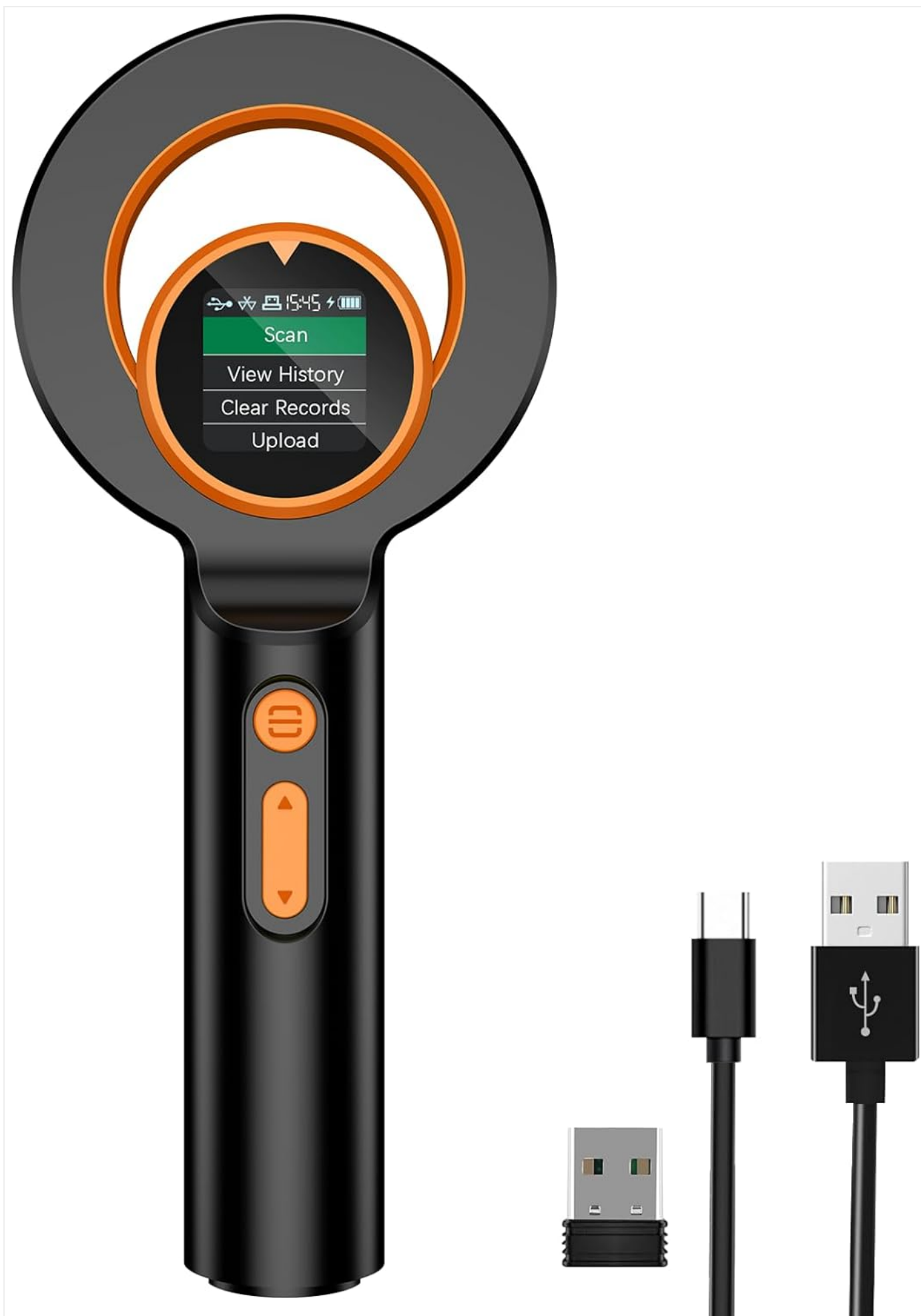
Image: The Alacrity Pet Microchip Scanner, showcasing its compact design, circular scanning head, and included accessories like the USB cable and 2.4GHz wireless dongle.
