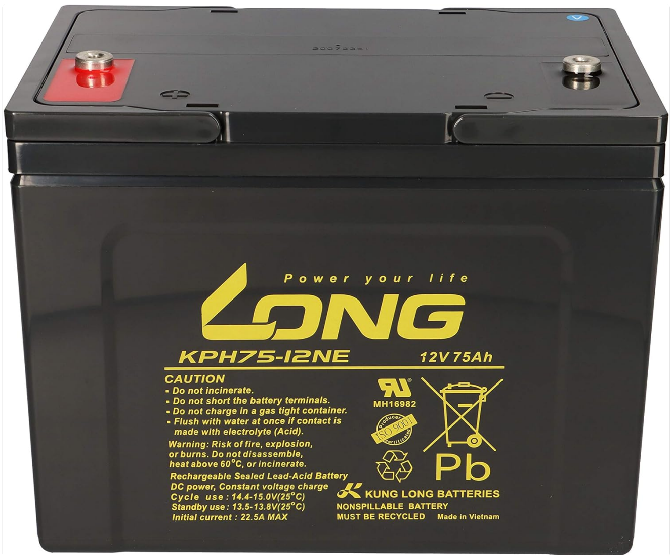
Image 2.1: Close-up of the product label on a Kung Long KPH75-12NE M6 12V 75Ah battery. The label includes critical safety warnings such as 'Do not incinerate,' 'Do not short the battery terminals,' and 'Risk of fire, explosion, or burns.' It also lists technical details like 'Rechargeable Sealed Lead-Acid Battery,' 'DC power, constant voltage charge,' 'Cycle use: 14.4-15.0V (25°C),' and 'Standby use: 13.5-13.8V (25°C). This information is crucial for safe handling and proper charging.
