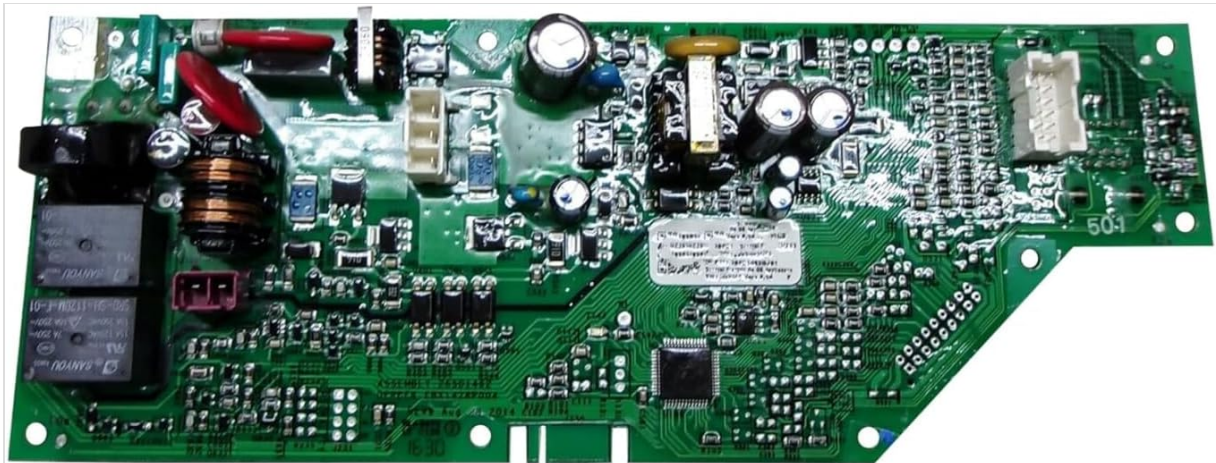
Image 1.1: Top view of the M93DVN Electronic Control Board, showing various electronic components, circuits, and connectors.
