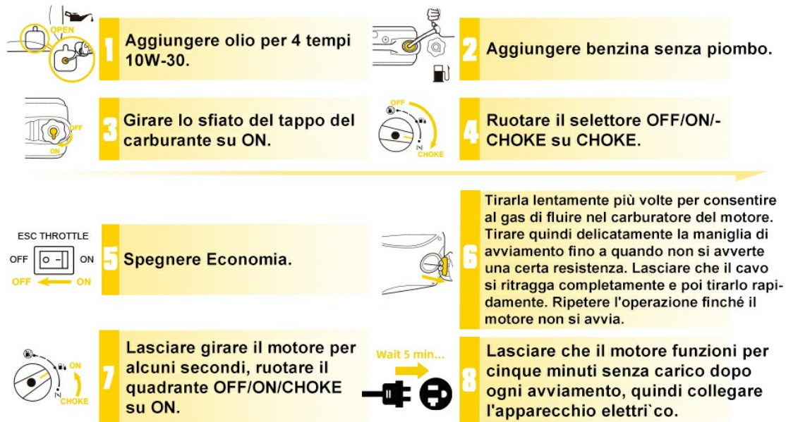
Figure 4.1: Engine Starting Steps. This diagram illustrates the 8-step process for starting the generator, including adding oil, adding fuel, turning the fuel cap vent to ON, setting the OFF/ON/CHOKE selector to CHOKE, turning off Economy mode, pulling the recoil starter, letting the engine run for a few seconds, and finally connecting electrical appliances after a 5-minute warm-up.
