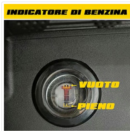
Figure 2.4: Fuel Gauge. A clear view of the fuel gauge, showing markings for "EMPTY" and "FULL" to indicate the fuel level in the tank.
