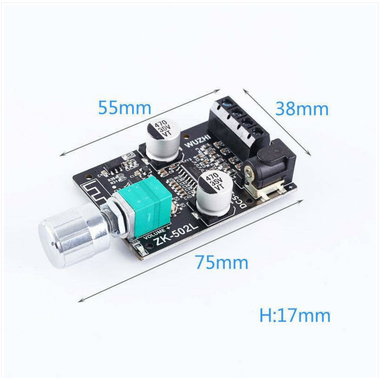
Figure 3.1: Physical dimensions of the ZK-502L module.
