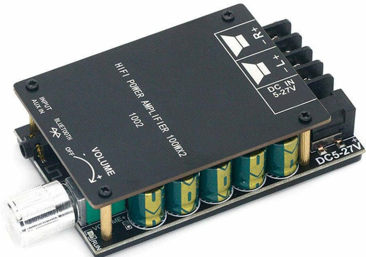
Front view of the ZK-1002 HiFi Digital Amplifier Board, showing the volume knob, input switch, and power/speaker terminals.
