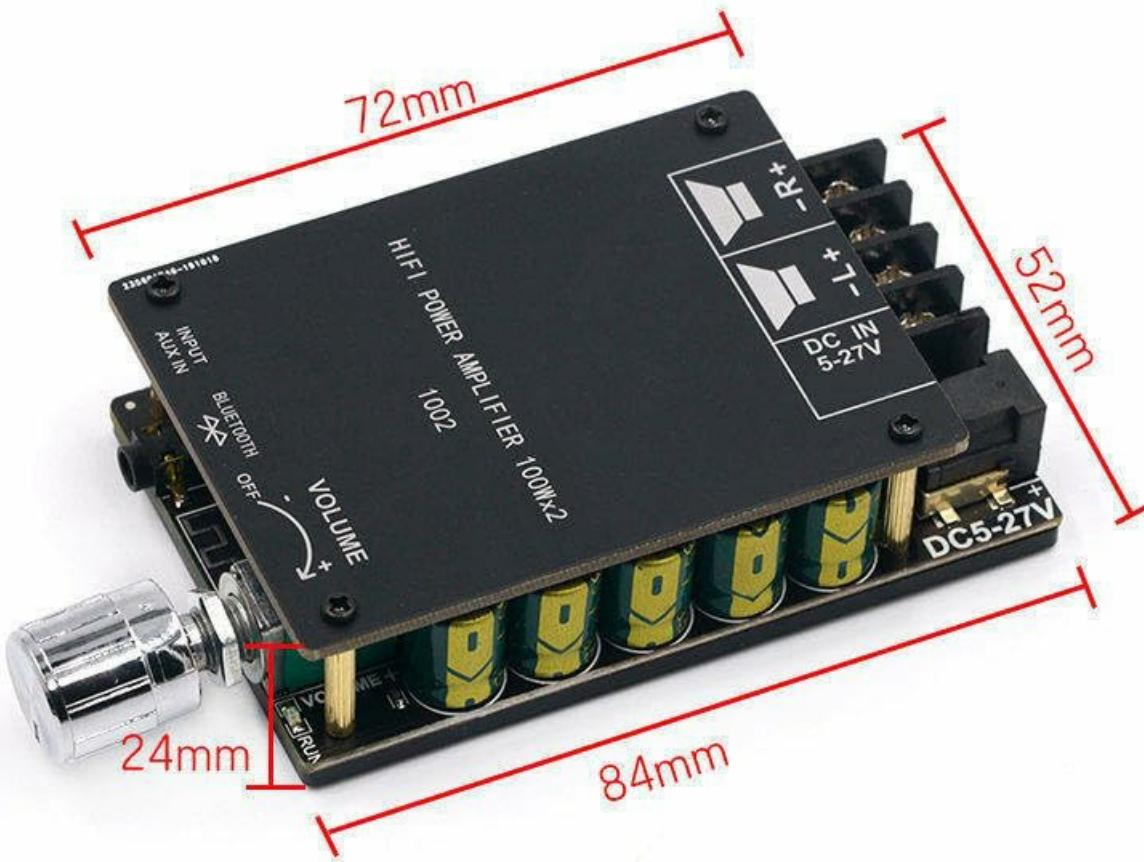
The ZK-1002 amplifier board with approximate dimensions indicated, showing its compact size.
