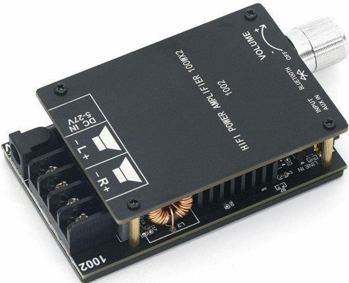
A detailed view of the ZK-1002 amplifier board, highlighting the DC power input and speaker output terminals for proper wiring.
