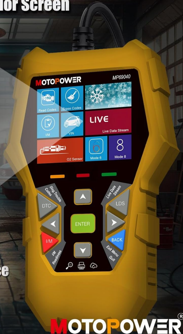
Figure 6.1: The user-friendly interface of the MP69040, featuring a 2.8-inch high-definition color screen with various diagnostic functions.
