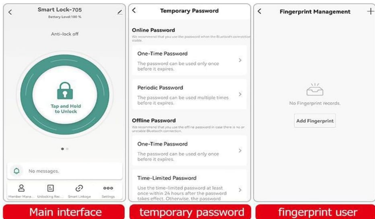
Figure 6: App interface for managing your smart lock, including temporary passwords and fingerprint users.
