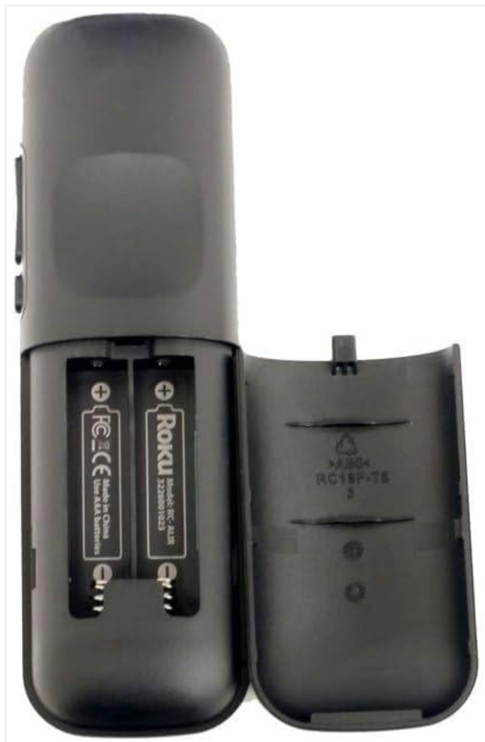
Figure 2: Back view of the remote control with the battery compartment cover removed, revealing the slots for two AAA batteries.
