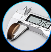
150mm/min 1pass cutting 9mm MDF
