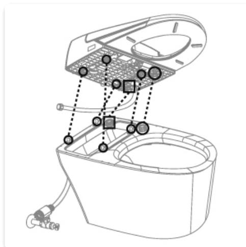
Image 4.2: Aligning the toilet with the floor bolts for secure placement.
