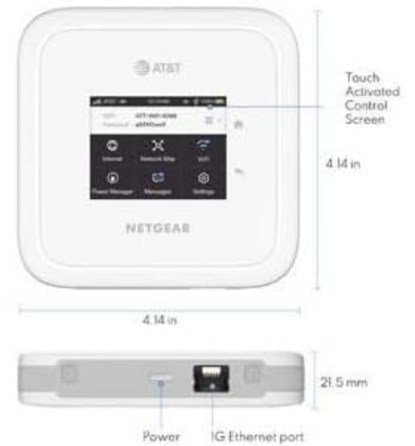
Image 3: Side view of the Nighthawk M6, highlighting the USB-C charging port and the Gigabit Ethernet port.
