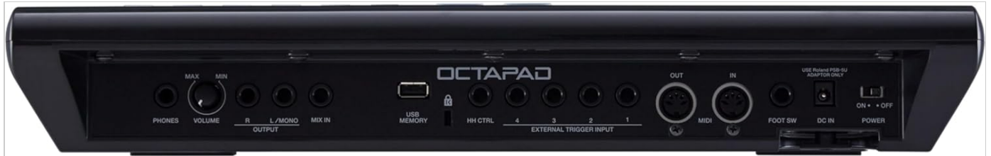
Image: Rear panel of the SPD-20PRO-BK, illustrating the power input, audio outputs, USB memory port, MIDI I/O, and external trigger inputs.
