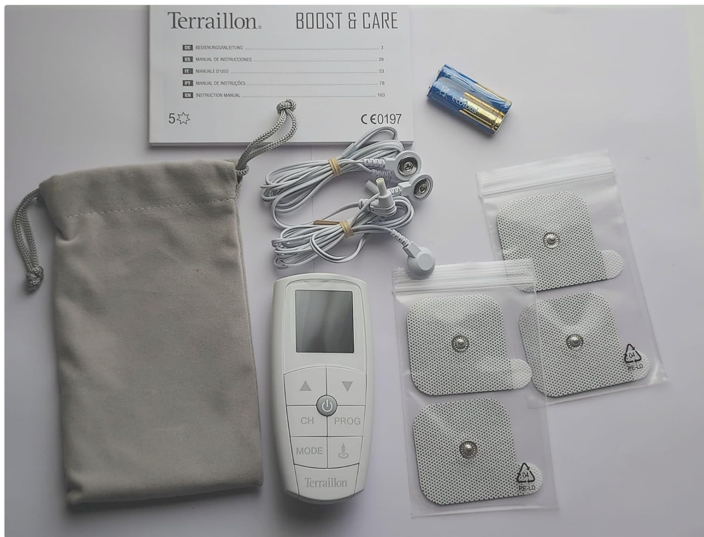
Figure 3.1: Package contents of the electro-stimulator. This image displays the main unit, electrode pads, connection wires, a storage pouch, and batteries.
