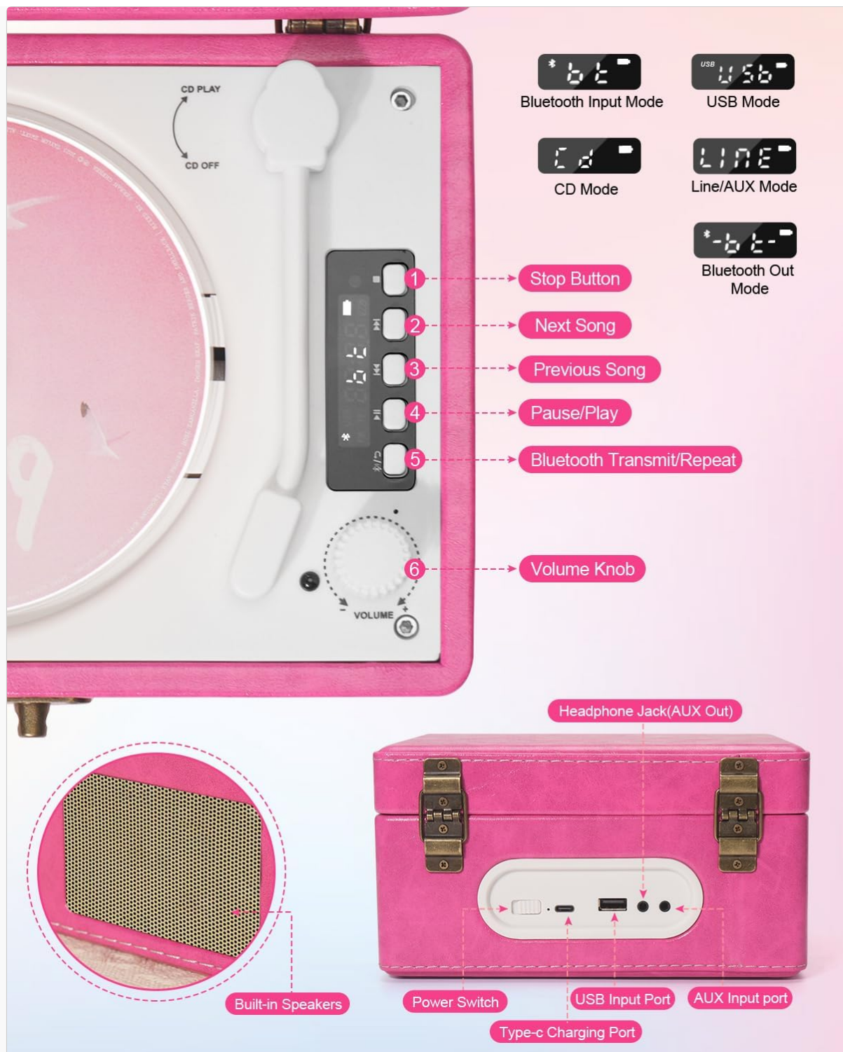
Figure 2.1: Front and rear view of the CD player, highlighting controls and ports. Key features include the CD play arm, control buttons (Stop, Next, Previous, Play/Pause, Bluetooth Transmit/Repeat), Volume Knob, Headphone Jack (AUX Out), Power Switch, USB Input Port, AUX Input Port, and Type-C Charging Port.
