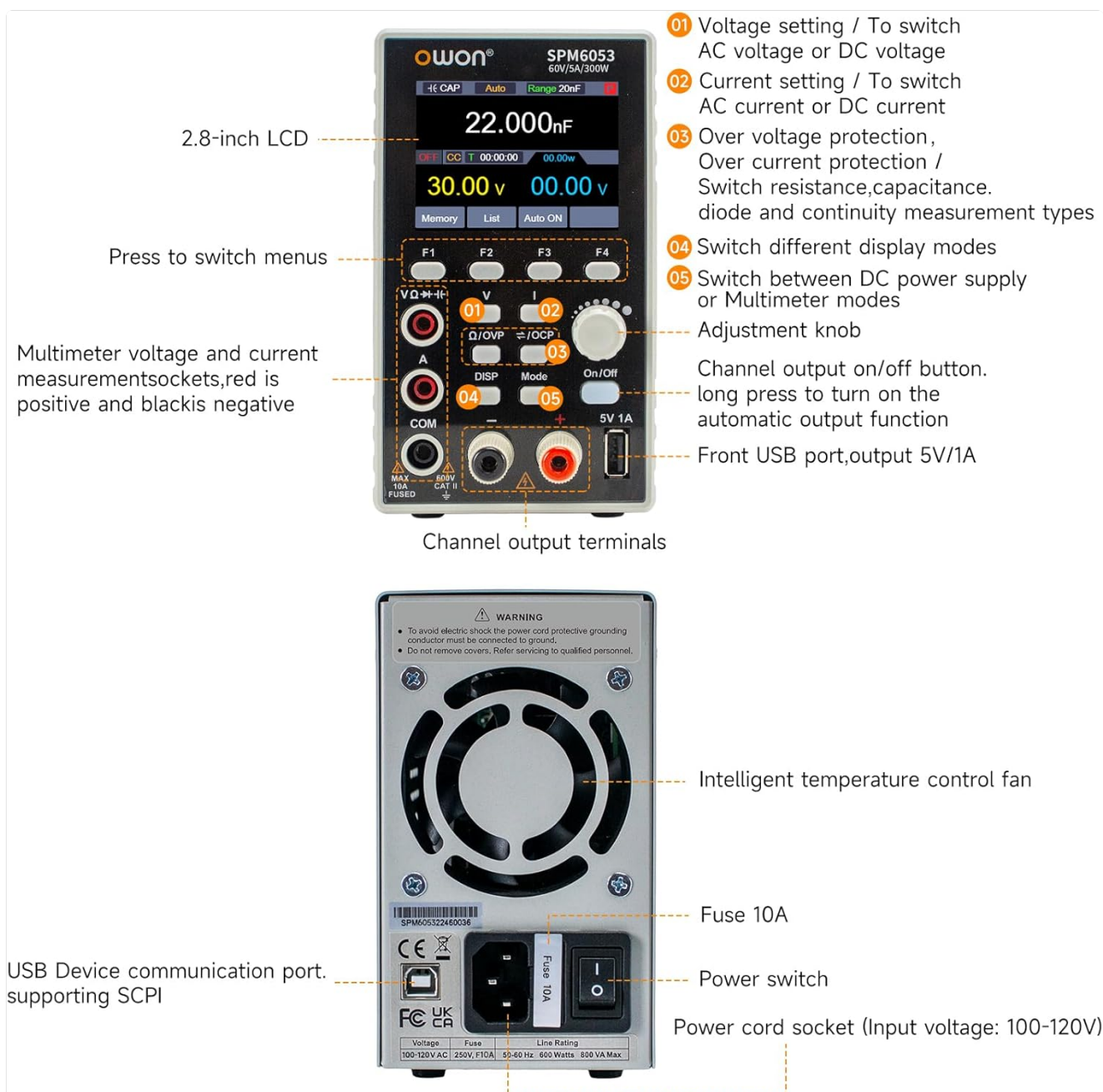
Figure 2.1: Front and rear panel overview. Note the power switch on the rear and the various input/output terminals on the front.
