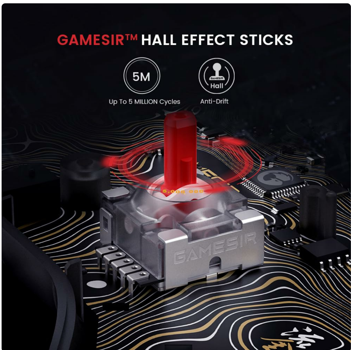
Image 5.1: Close-up view of the GameSir Hall Effect stick mechanism, illustrating its anti-drift and high durability (up to 5 million cycles) features.
