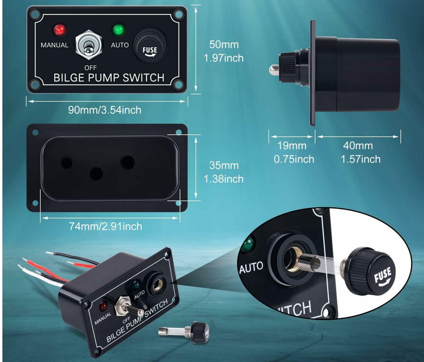
Figure 1: Product dimensions and replaceable fuse location. The panel measures approximately 90mm (3.54 inches) wide by 50mm (1.97 inches) high on the front face. The rear housing is approximately 74mm (2.91 inches) wide by 35mm (1.38 inches) high, with a depth of 40mm (1.57 inches) from the mounting surface. A 5A fuse is integrated and accessible for replacement.
