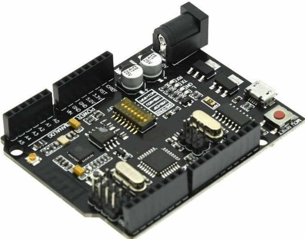
Figure 1: Top-down view of the Generic WiFi R3 ATmega328P+ESP8266 Development Board, showing various components and pin headers.
