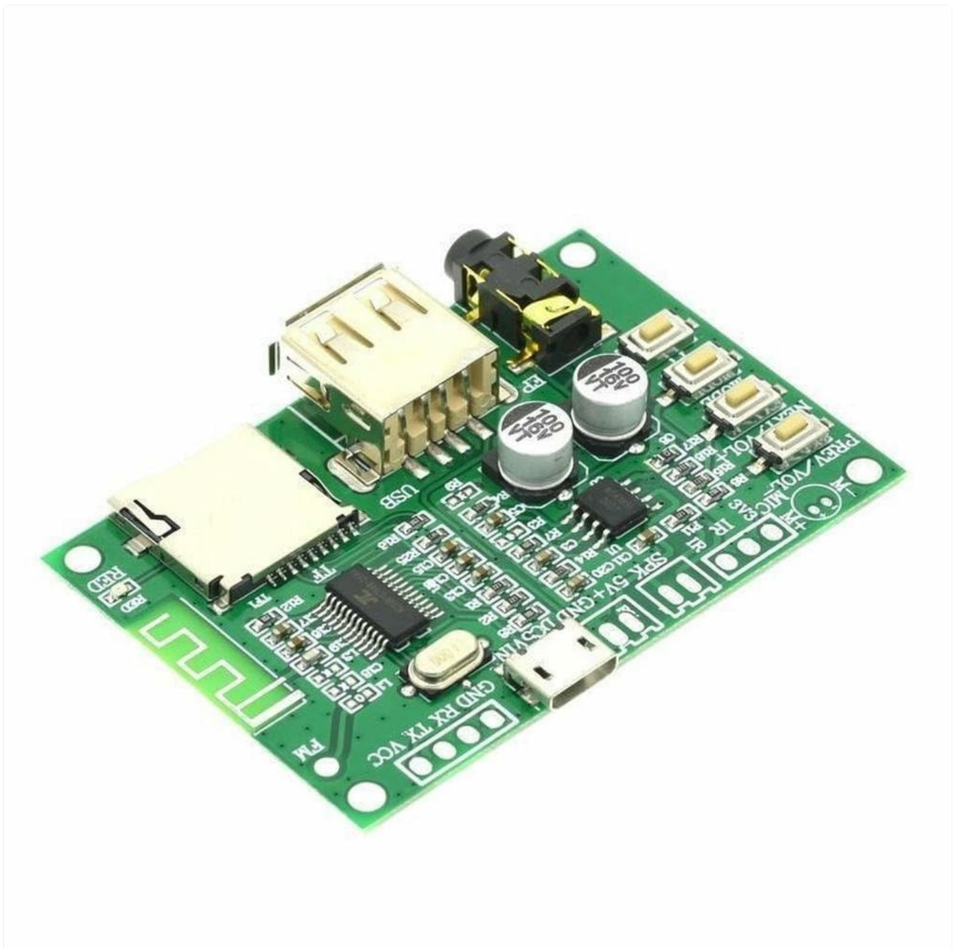
Figure 3.2: Angled view of the BT201 module. This perspective provides a clearer look at the USB host port and the TF card slot, essential for media playback.
