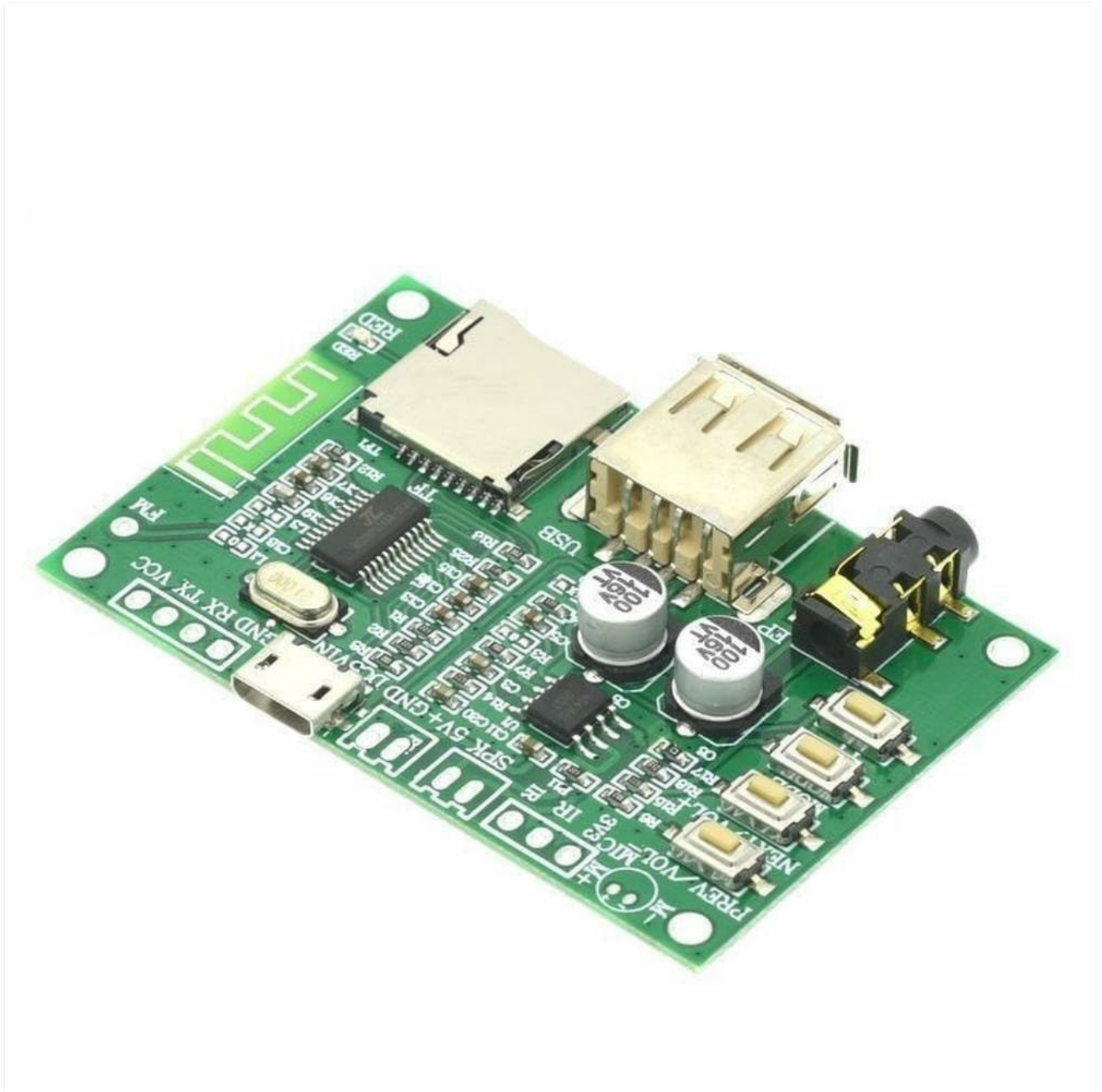
Figure 3.1: Top view of the BT201 module. This image displays the main components including the USB port, TF card slot, audio jack, and control buttons. Key connection pins for power, ground, and data are also visible.
