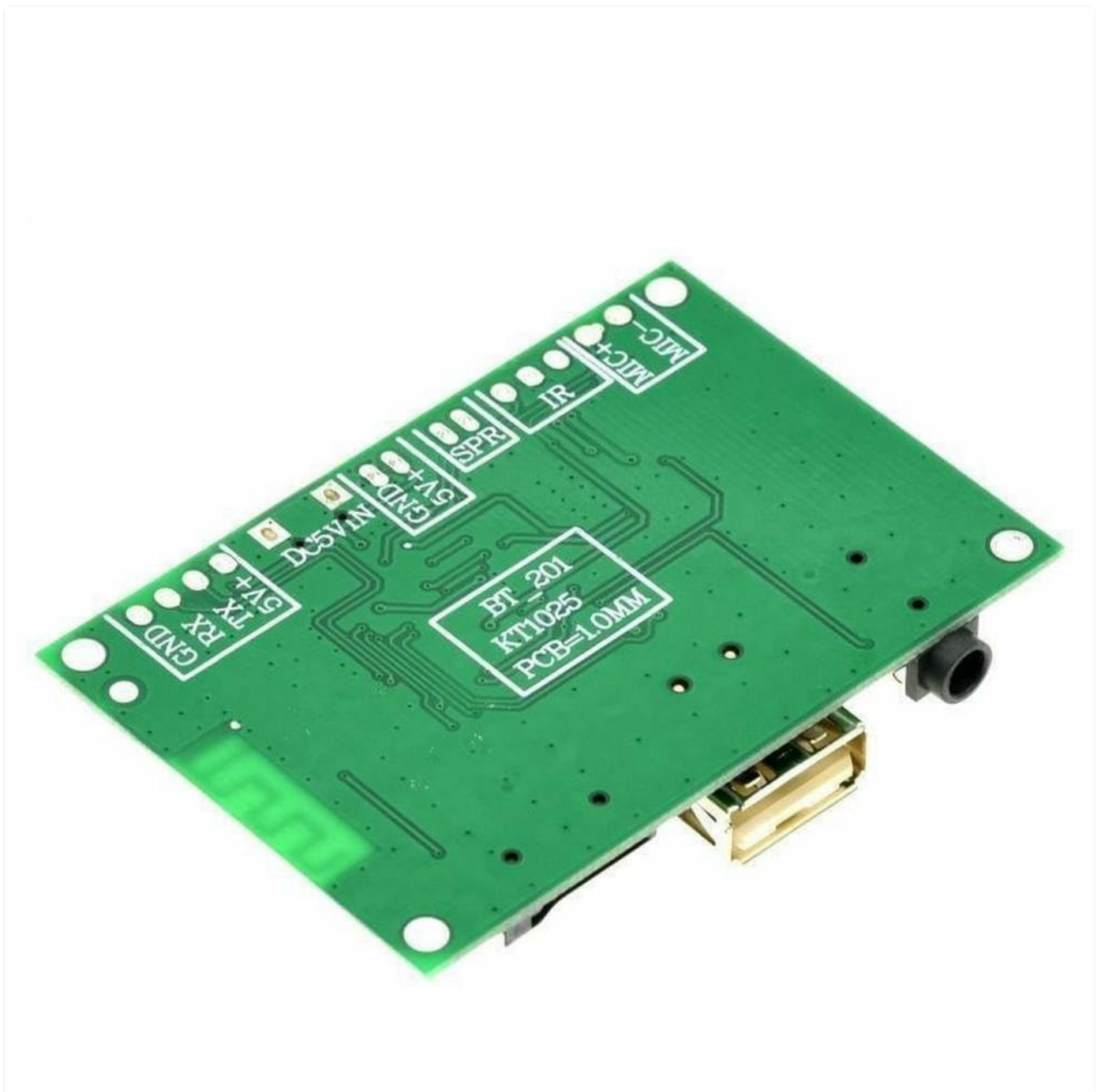
Figure 3.3: Bottom view of the BT201 module. This image shows the printed circuit board (PCB) traces and the model designation "BT201 KT1025" printed on the board.
