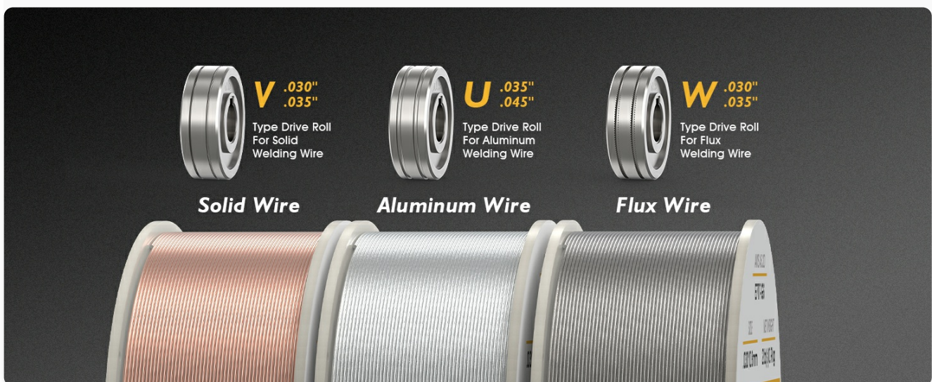
Figure 5: Different drive roll types for Solid, Aluminum, and Flux wires.
