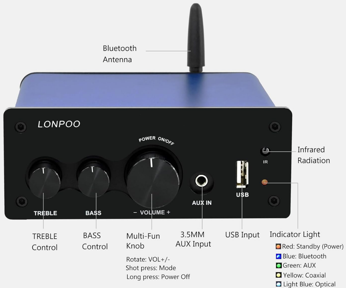
Image 2.1: Front panel layout of the LONPOO AMP-615 amplifier. This image displays the Treble control, Bass control, Multi-Function Volume knob (rotate for volume, short press for mode, long press for power off), 3.5mm AUX Input, USB Input, Infrared (IR) receiver, and indicator light.
