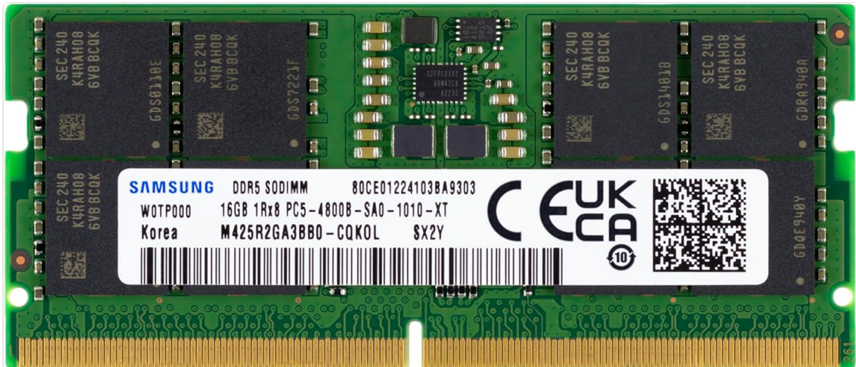
Image 1.1: Front view of the Samsung 16GB DDR5 SODIMM RAM module. The module features multiple black memory chips on a green circuit board, with a white label displaying "SAMSUNG DDR5 SODIMM", "16GB 1Rx8 PC5-4800B", and the model number "M425R2GA3BB0-CQKOL".
