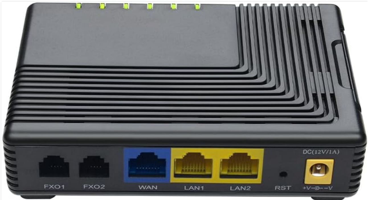
Figure 3: Rear panel of the FTA5120 showing FXO1, FXO2, WAN, LAN1, LAN2, RST, and DC 12V/1A ports.
