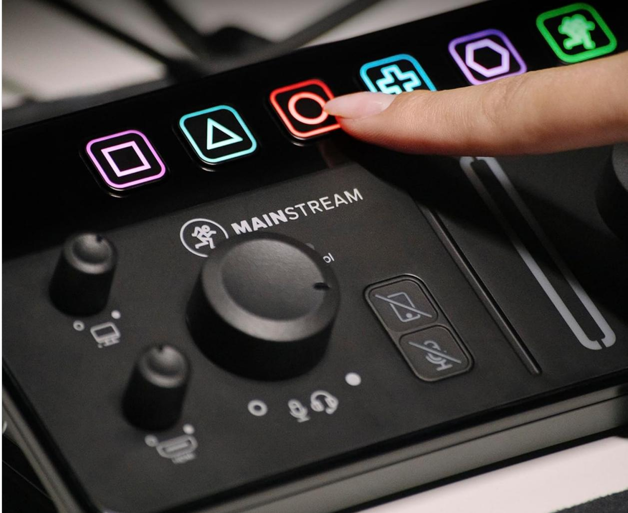
The six programmable keys can be customized to trigger samples or transitions.
