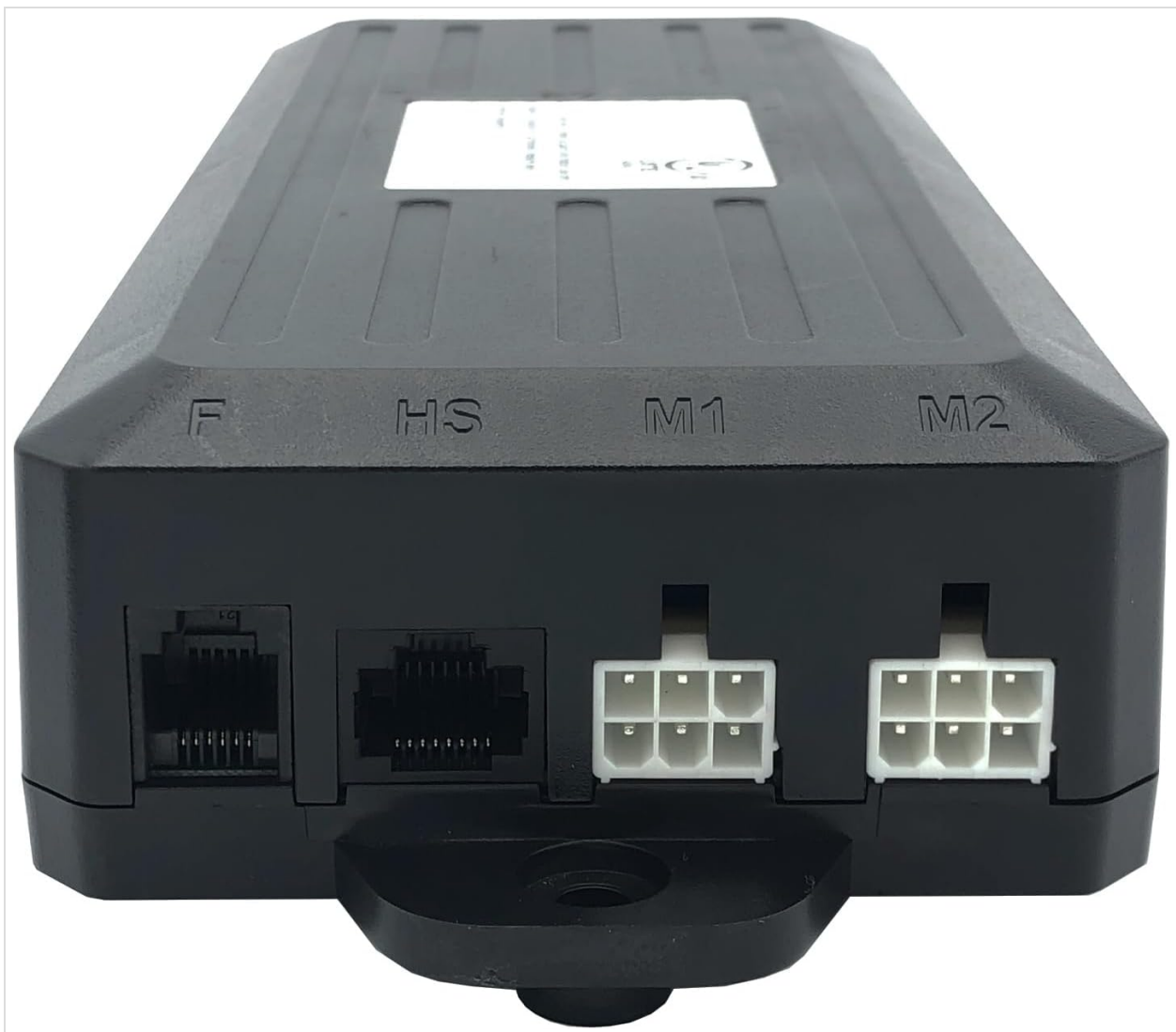
Figure 5.2: Output ports for linear actuators (M1, M2) and handset (F, HS).
