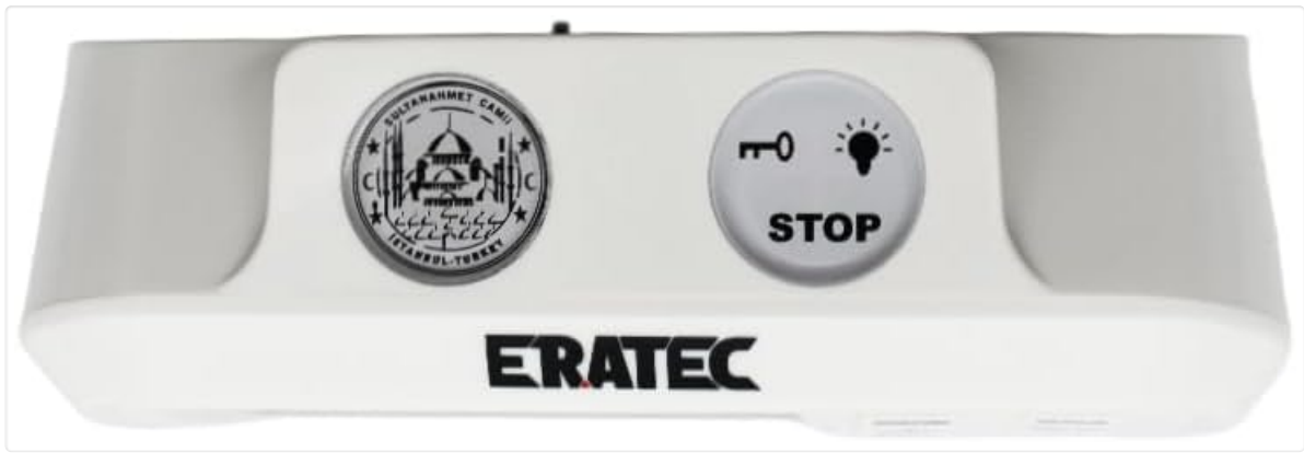
Figure 2.3: Top View of ERATEC AZ-6500. This image shows the top panel of the clock, featuring a 'STOP' button (likely for alarms/Azan) and a button for display backlight or light function.
