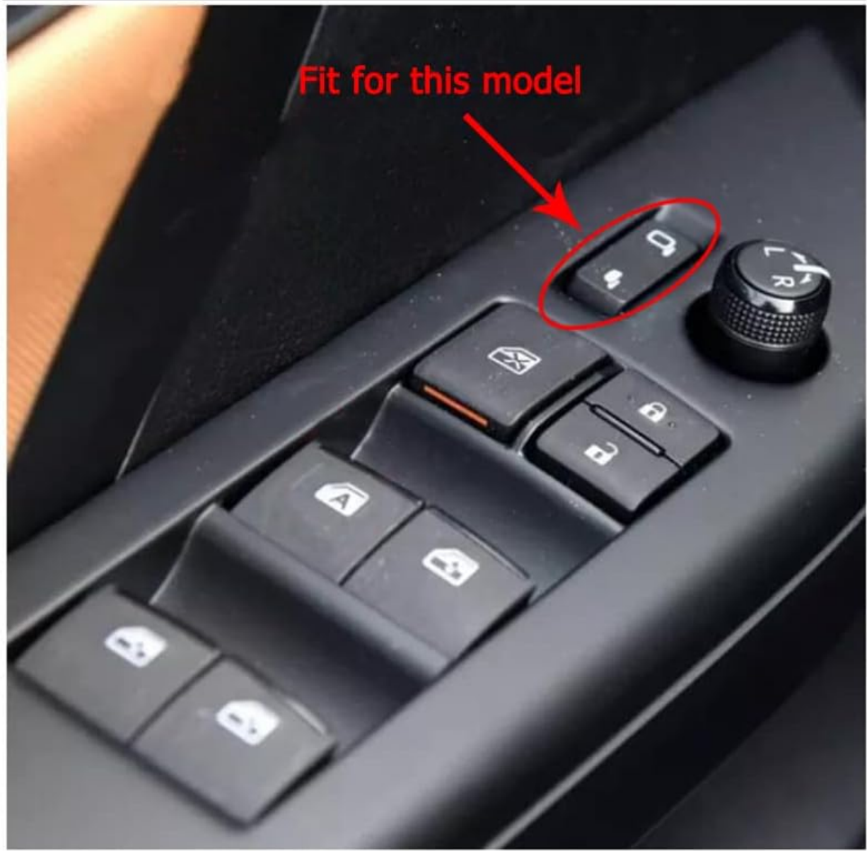
Image 3.1: Example of a compatible vehicle's automatic mirror folding button.
