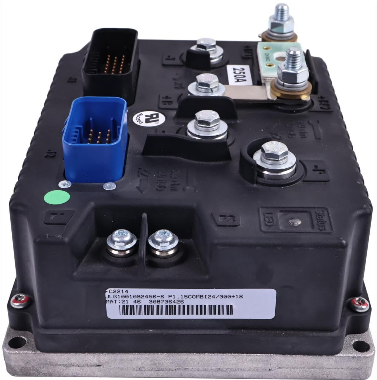
Figure 2: Top view of the control module, showing various terminals, connectors, and a label with the part number "JLG1001092456" and other identification details. A 250A fuse rating is also visible.
