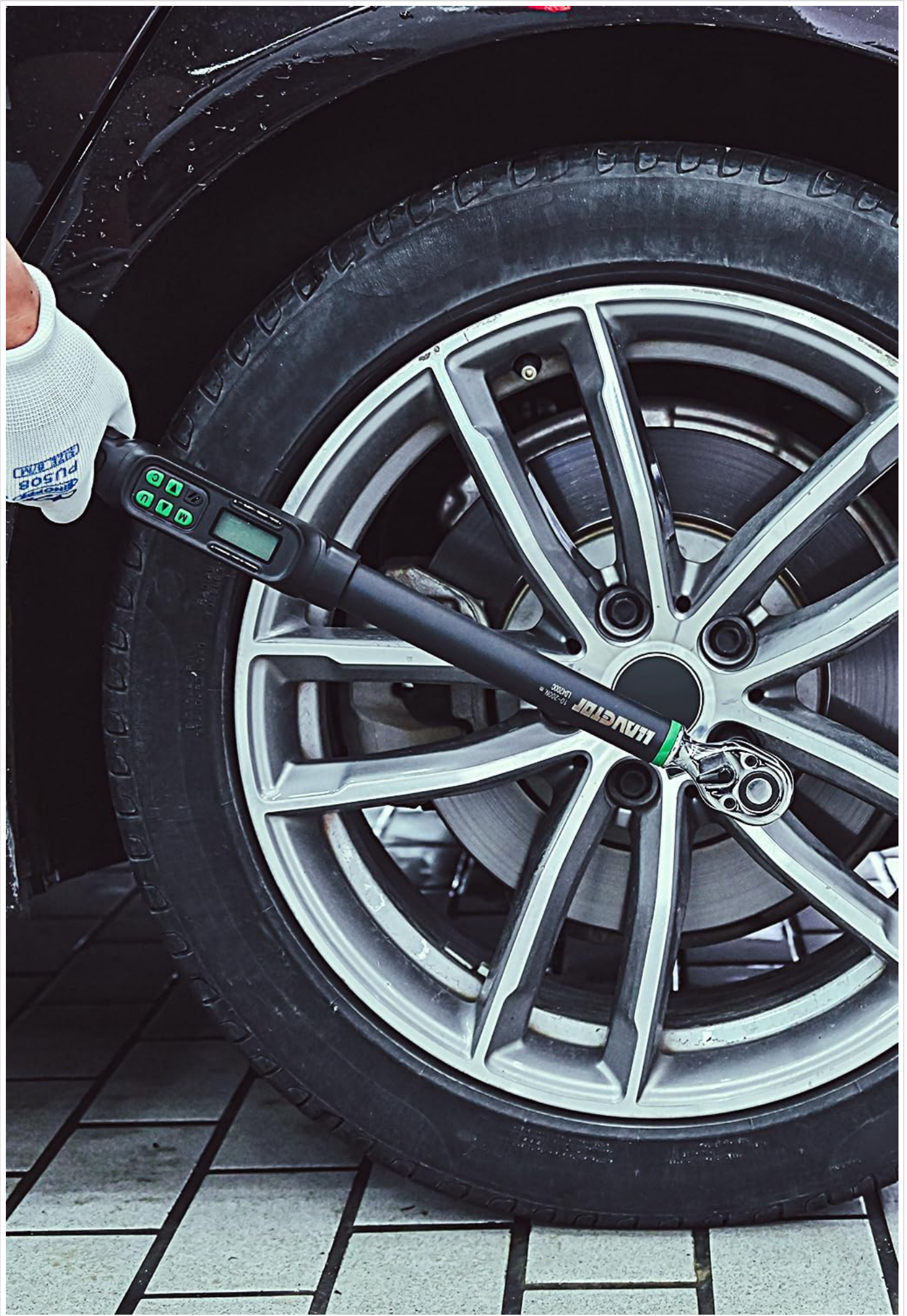
Figure 7: The LLAVETOR Digital Torque Wrench being used to tighten lug nuts on a car wheel, demonstrating a typical application.
