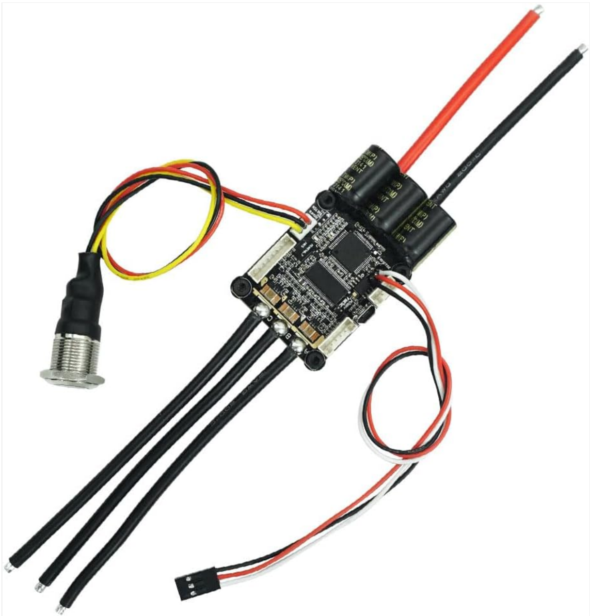
Figure 3.2: Top view of the ESC, highlighting the main integrated circuits, capacitors, and various connection ports.
