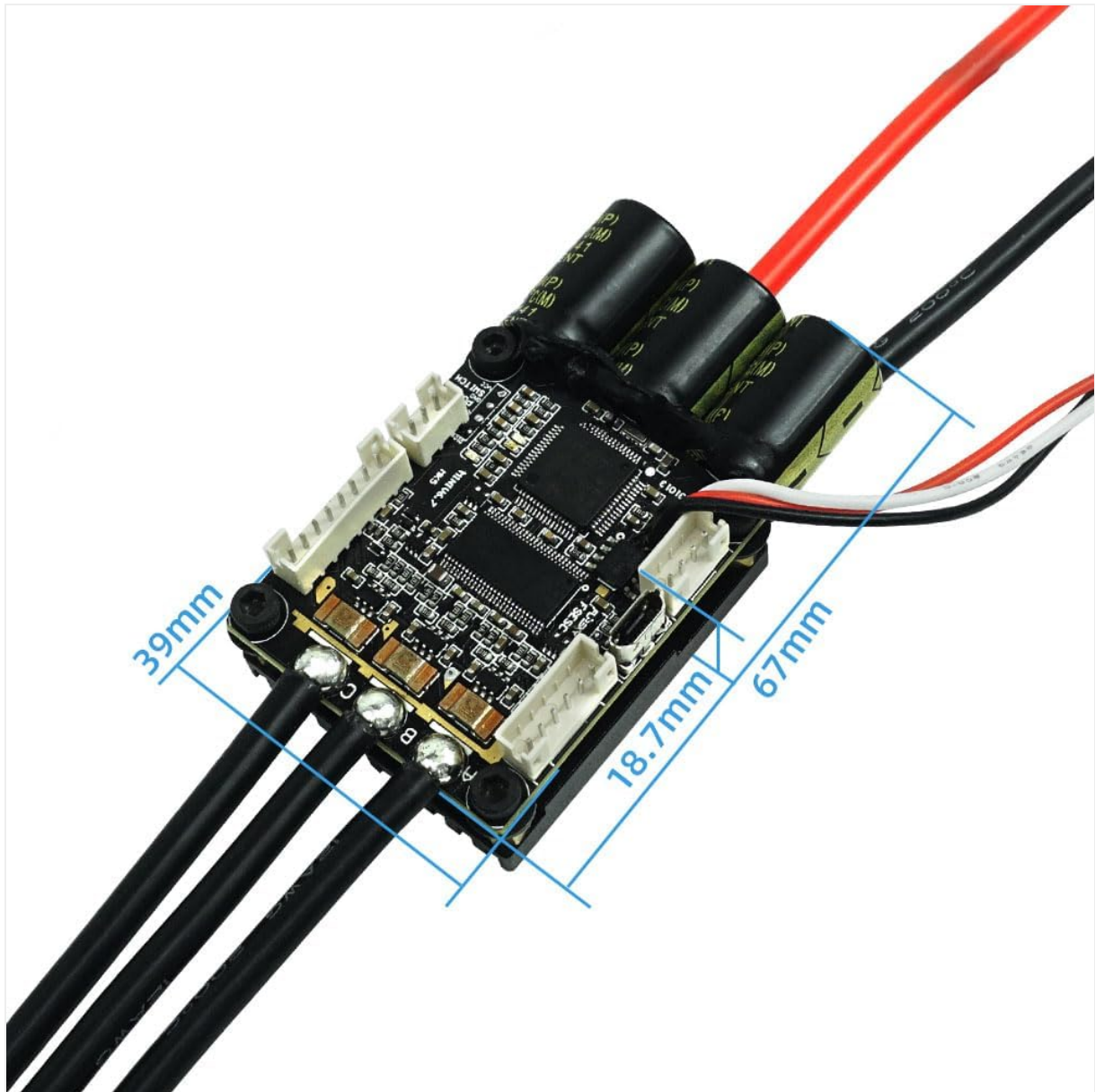
Figure 4.1: Dimensions of the FLIPSKY Mini V6 MK5 ESC, showing length, width, and height measurements.
