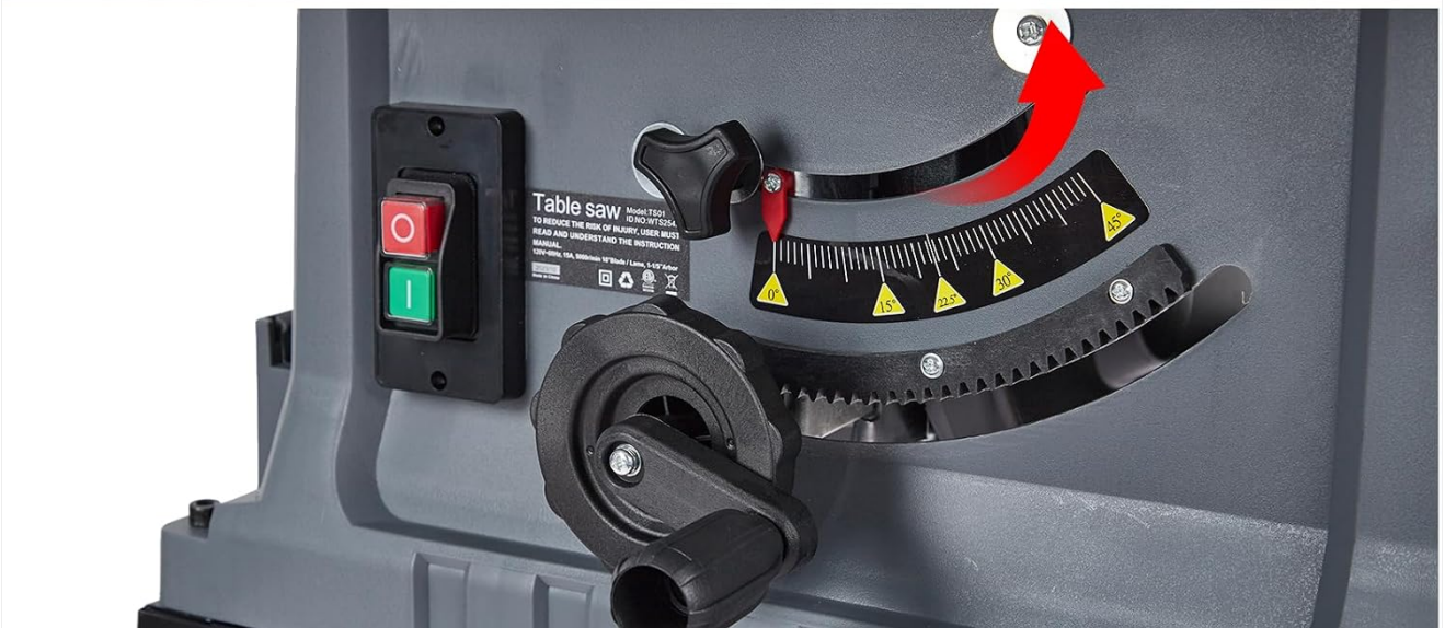
Image: Close-up of the hand wheel mechanism for adjusting the blade height on the Garvee Table Saw.
