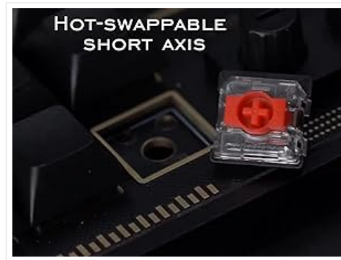
Close-up of a hot-swappable short axis switch on the NLOFIN KB16 macro pad.
