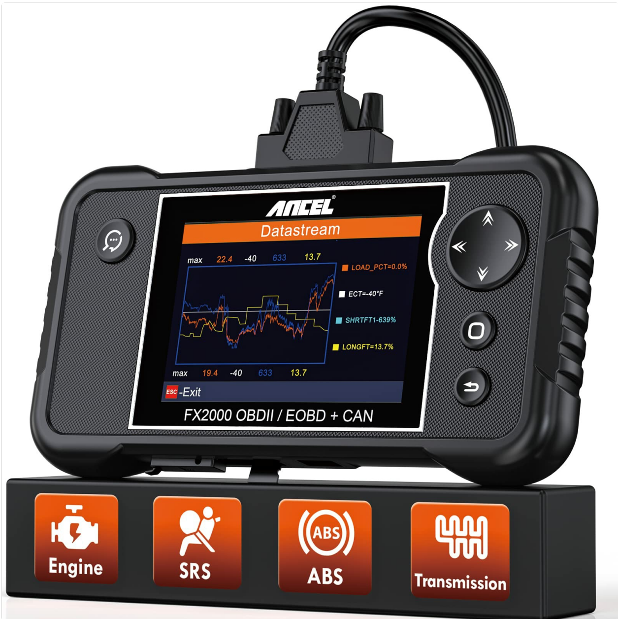
Figure 2.2: ANCEL FX2000 displaying live data and system icons.
