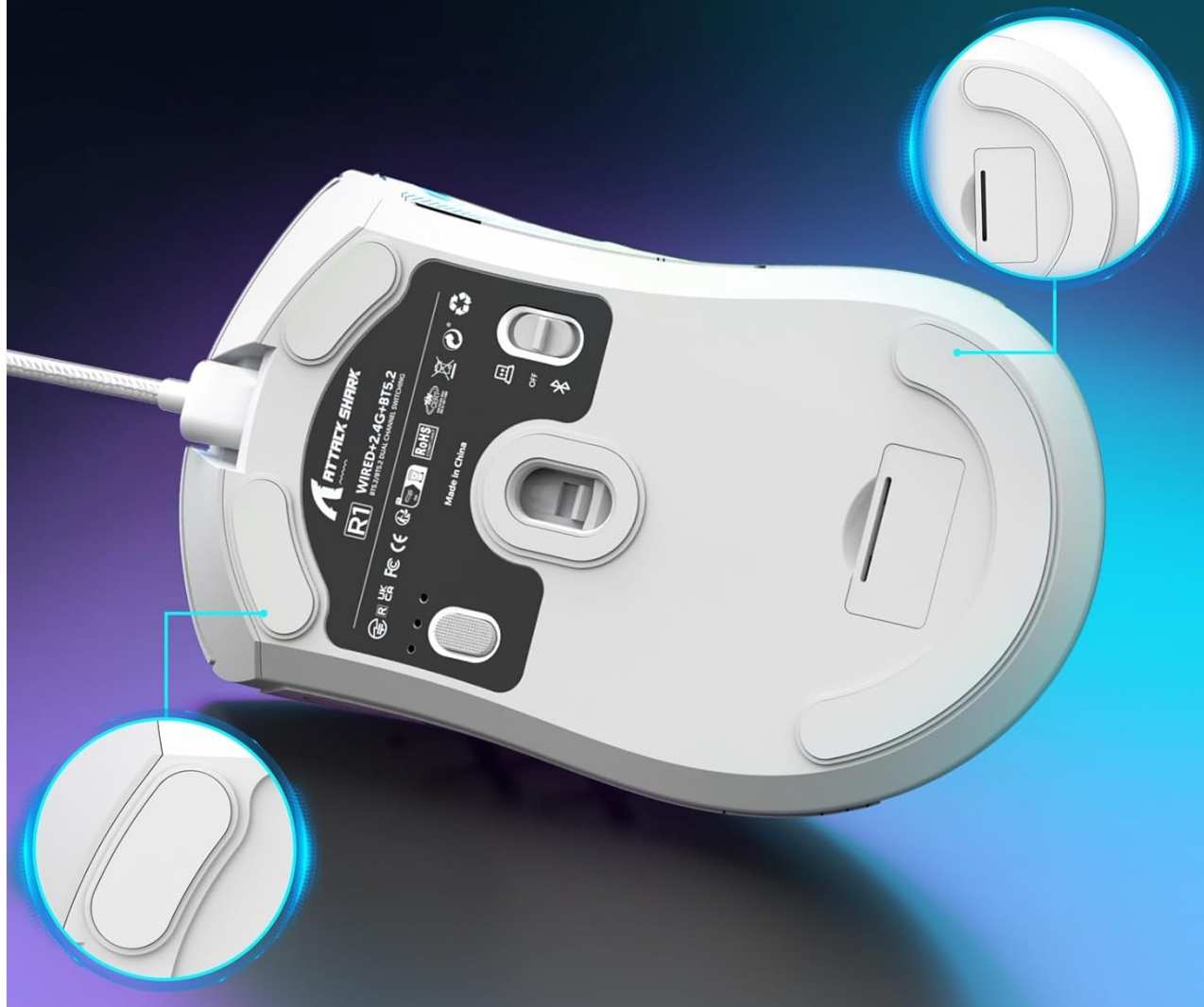
Figure 7: The underside of the mouse, featuring high-strength, low-friction anti-slip foot pads for smooth gliding, along with the connection mode switch and a compartment for the USB receiver.
