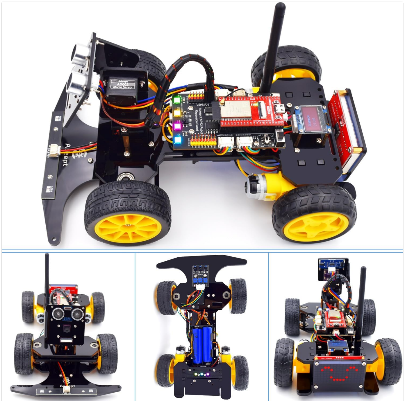
Image: A collage illustrating the diverse functionalities of the Adept Smart Car, including control via IR remote, autonomous obstacle avoidance, following a line, displaying information on the OLED screen, showing patterns on the LED matrix, streaming video, tracing light, and illuminating with WS2812 RGB LEDs.
