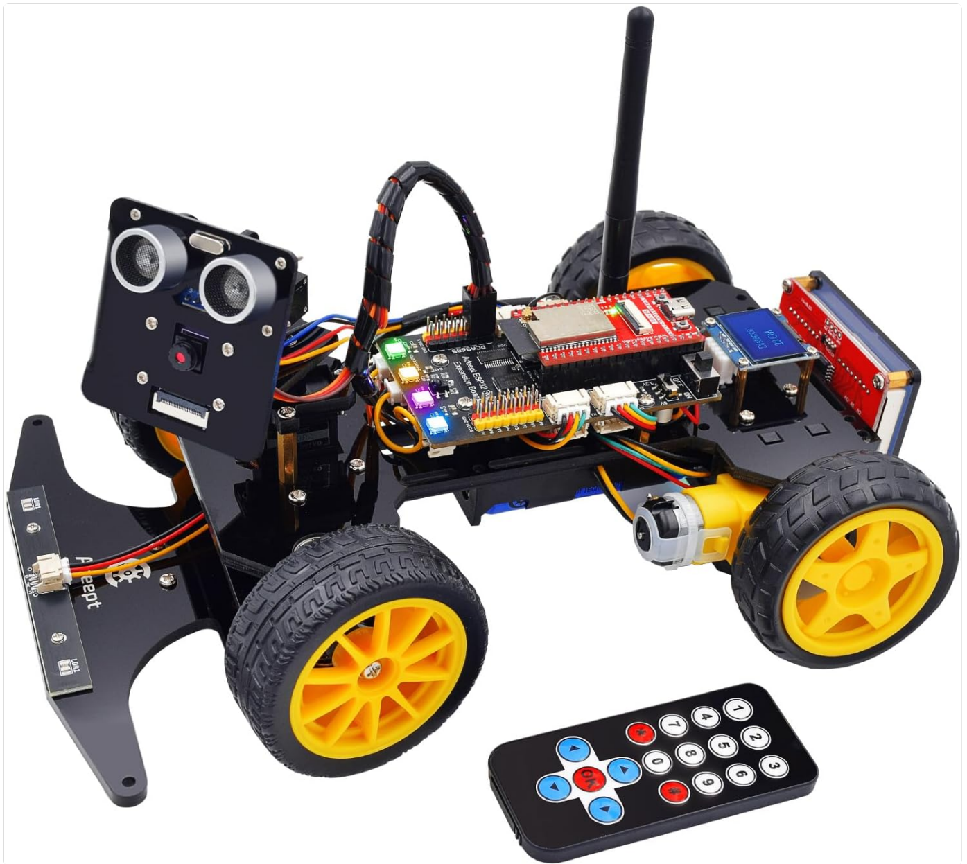
Image: The fully assembled Adept Smart Car Kit, showcasing its compact design and included remote control. The car features an ultrasonic sensor at the front and an ESP32-WROVER board with various modules mounted on its chassis.
