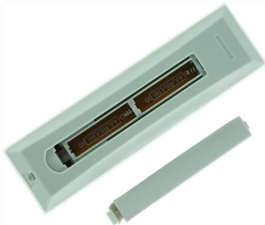
Image: Back of the remote control with the battery compartment open, illustrating where to insert two AAA batteries. Observe the polarity markings.
