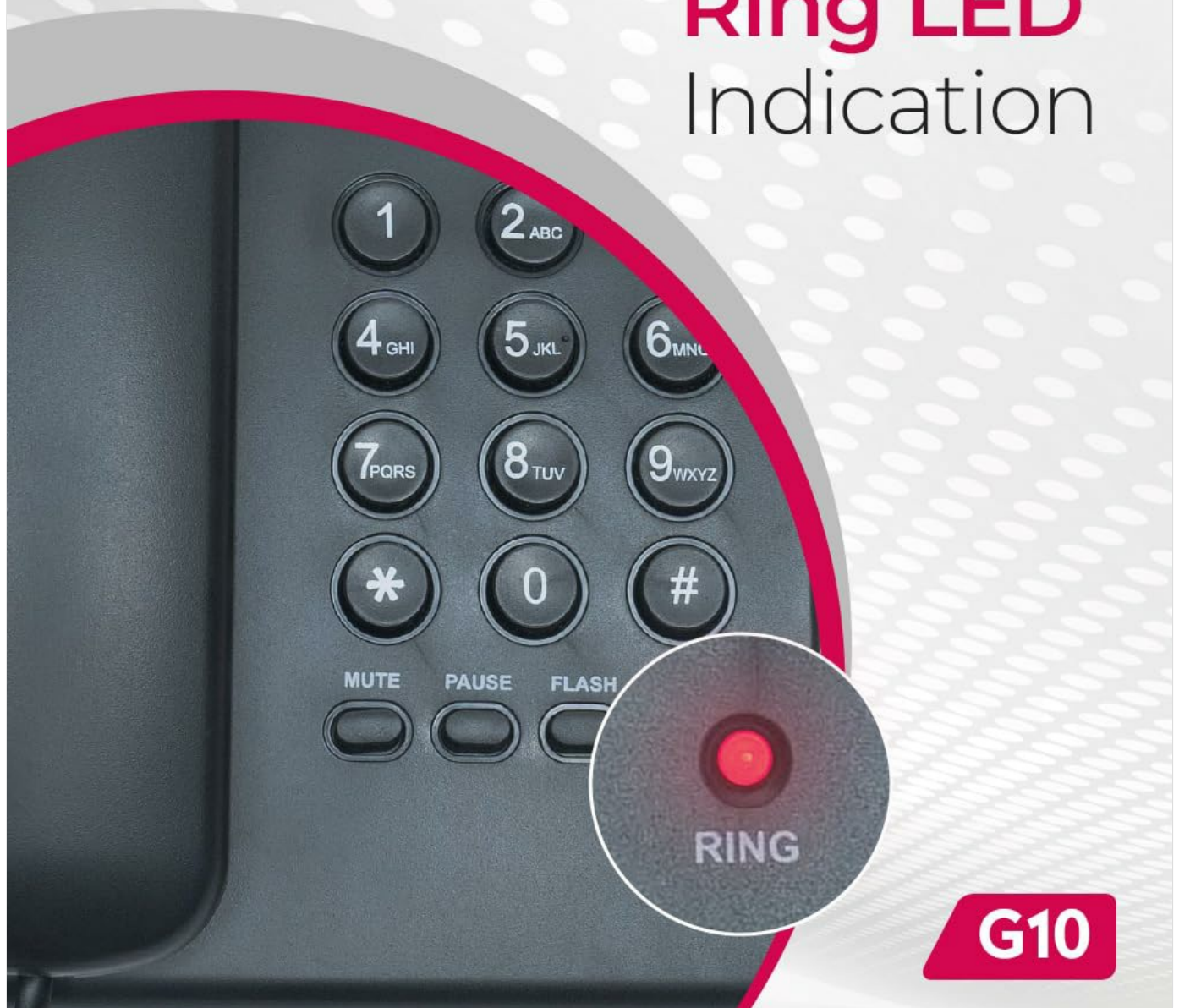
Figure 4.2: Front view of the Beetel G10 phone, specifically highlighting the Ring LED Indication. This LED illuminates when there is an incoming call, providing a visual alert.
